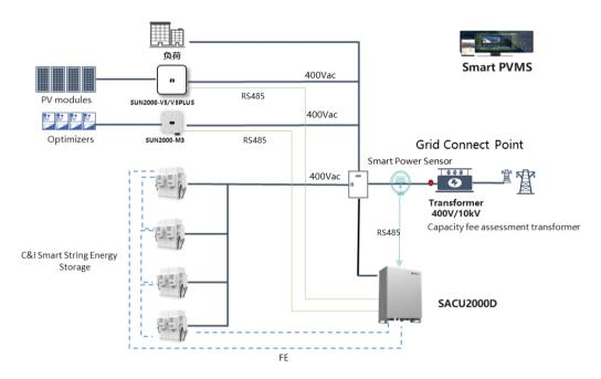
Huawei C&I Smart String Energy Storage (ESSs for short) Products LUNA2000B series are applicable to industrial and commercial scenarios. They work with the SmartPCS, DCDC and SACU. The SmartPCS is connected to the pack controller DCDC, and charges batteries when the power grid is sufficient. When the power grid needs to be output, the SmartPCS outputs the stored battery energy to loads for use.
