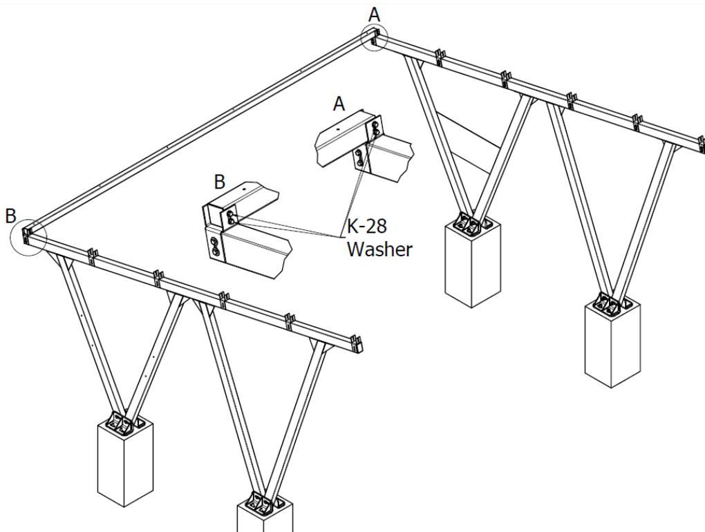
Figure 15. Installation of the W-02-06 beams, projection II
