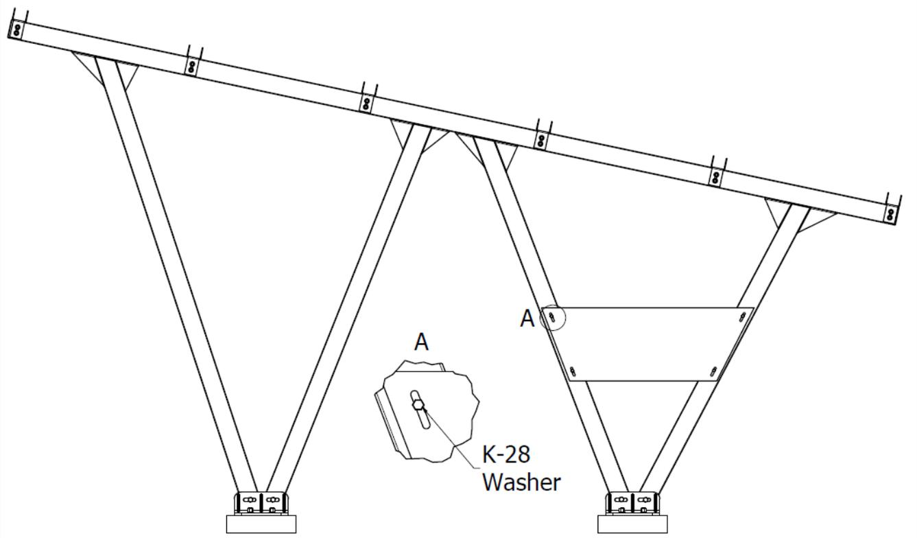
Figure 12. W-02-18 element assembly
