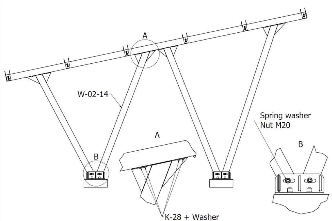
Figure 11. Installation of the W-02-14 support, projection II
