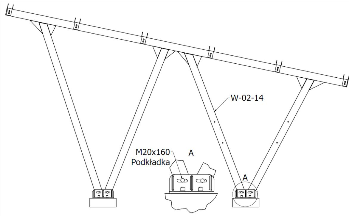
Figure 10. Installation of the W-02-14 support, projection I
