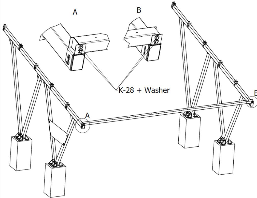
Figure 14. Installation of the W-02-06 beams, projection I
