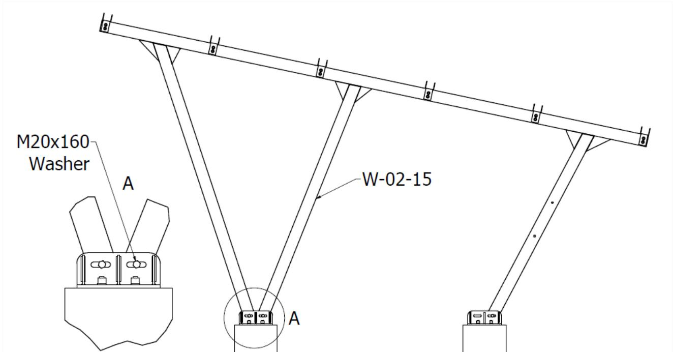
Figure 8. Installation of the W-02-15 support, projection I
