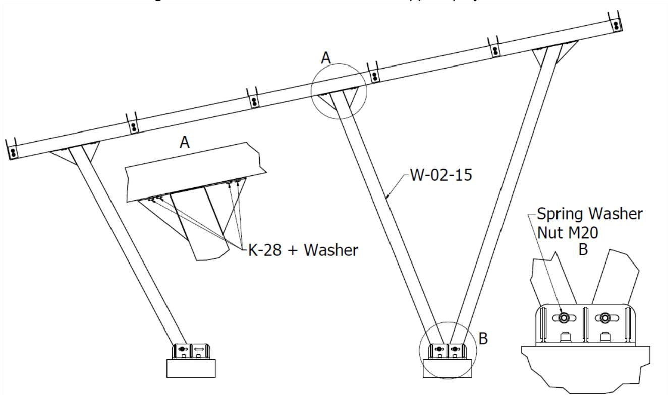
Figure 9. Installation of the W-02-15 support, projection II
