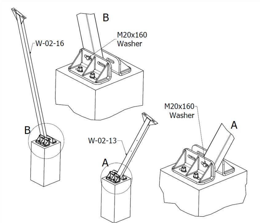
Figure 5. Preliminary installation of the W-02-16 and W-02-13 supports, projection I
