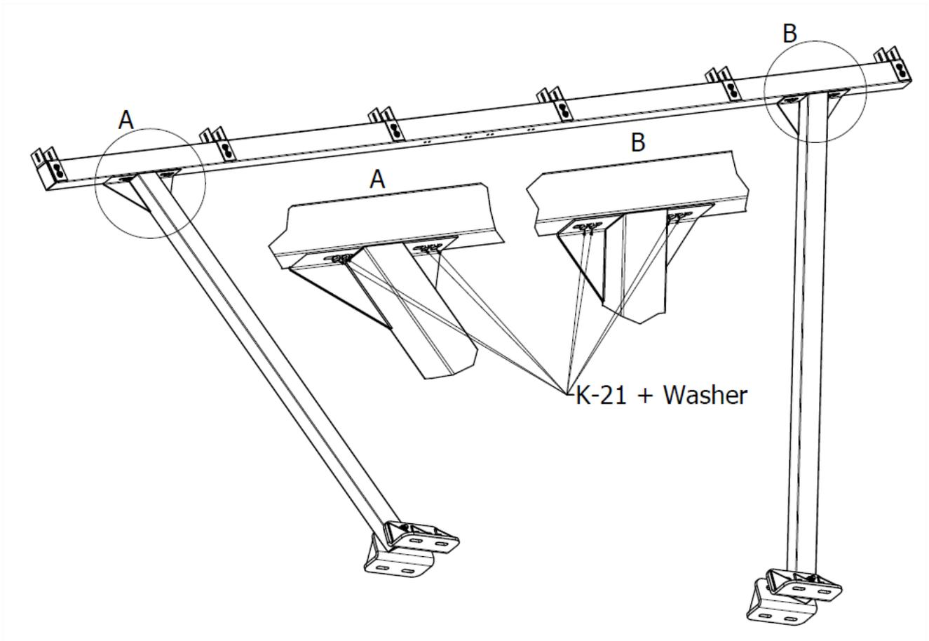
Figure 7. Pre-assembly of rafters to supports
