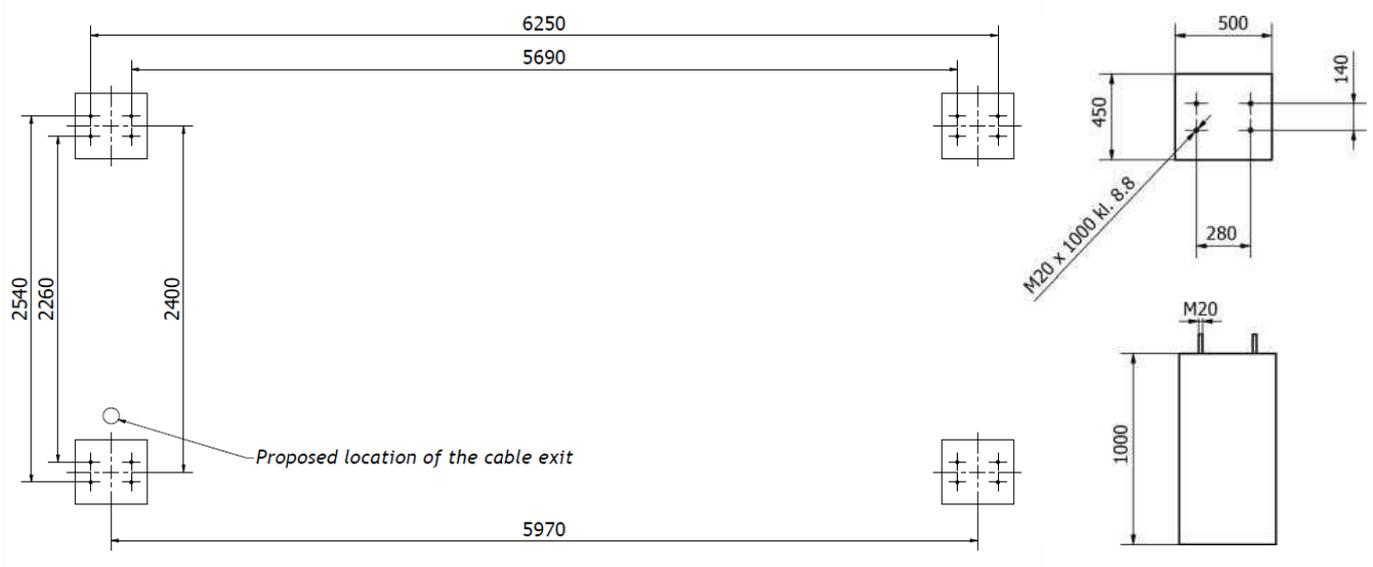
Figure 1. Layout of foundations
