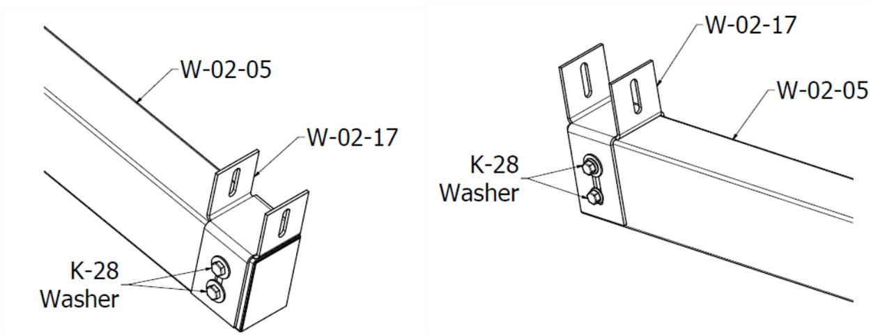
Figure 4. Installation of the W-02-17 elements on rafters
