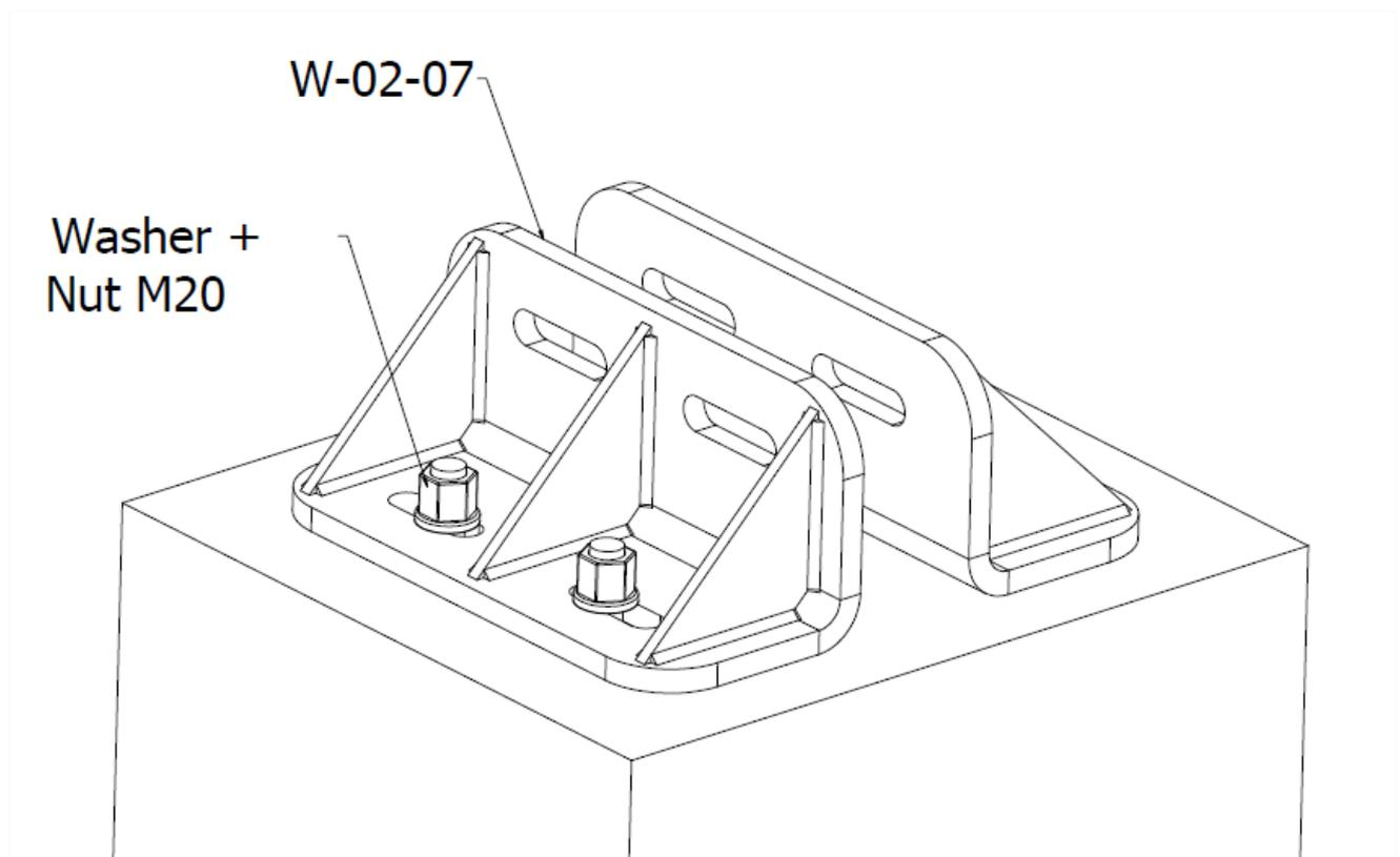
Figure 2. Initial bolting of the foundation sheet
