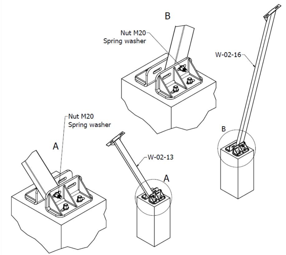
Figure 6. Preliminary installation of the -02-16 and W-02-13 supports, projection II
