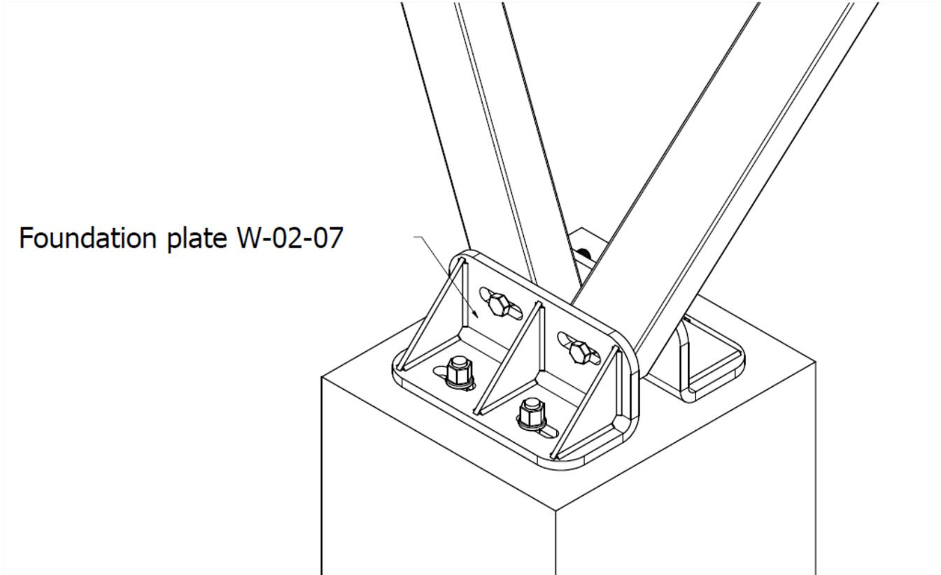
Figure 16. Tightening of foundation plates
