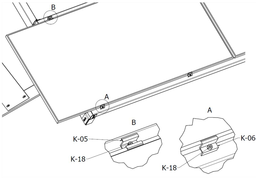
Figure 18. Installation of clamps
